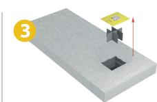
Remove the RÉZABOITE CV top-cover and strengtheners.
